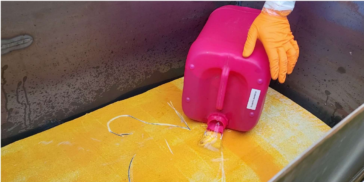
Figure 5: The H 2 O 2 is poured manually into the reaction chamber
