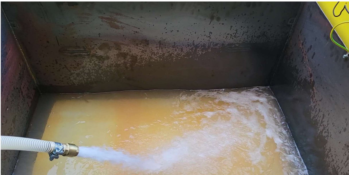
Figure 6: The acetic acid is injected without human presence via a dedicated inlet
