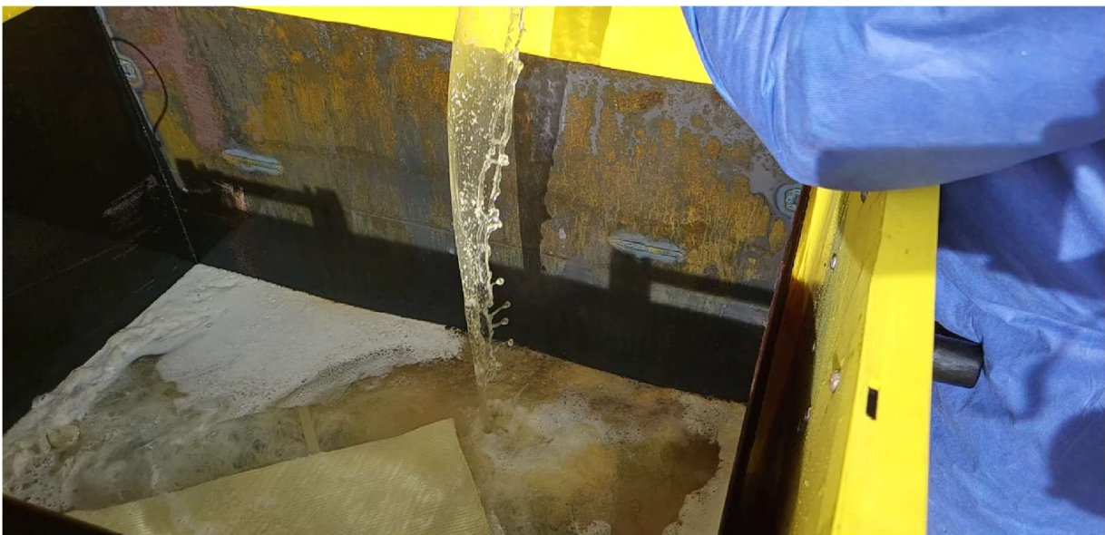
Figure 10: NaOH is poured manually into the emptied reactor to neutralize residual PAA that is absorbed within the blade fragment
