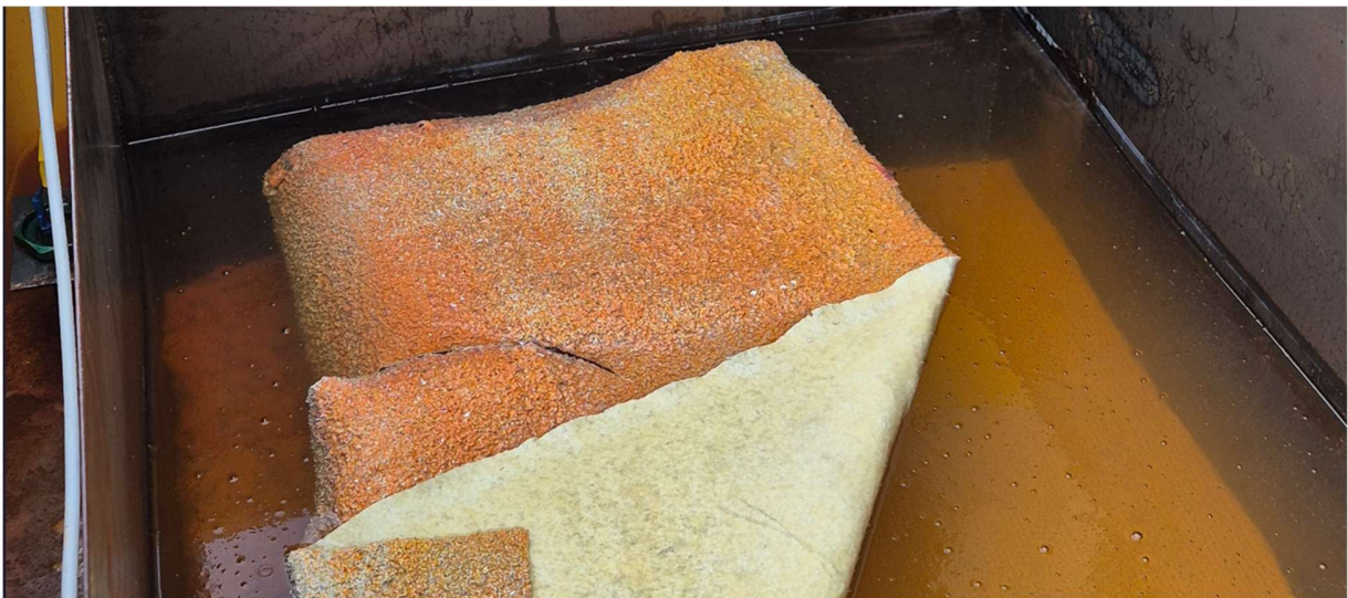
Figure 8: After 6 hours, the de-laminated coating (1 st layer of the fragment) is visible on the surface of the reactor
