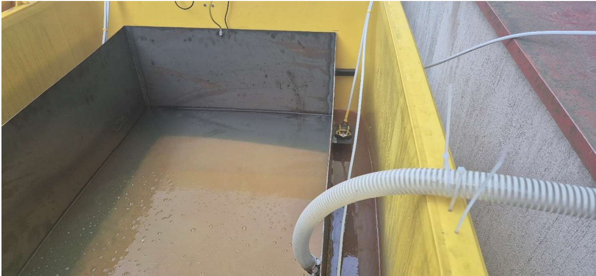
Figure 7: The reaction begins. ~250L of water is heated to 55C thus heating 215L of PAA to the same temperature. PAA and water vapor condenses on the reactor wall. Reaction bubbles emerge immediately upon contact with epoxy and coating surface
