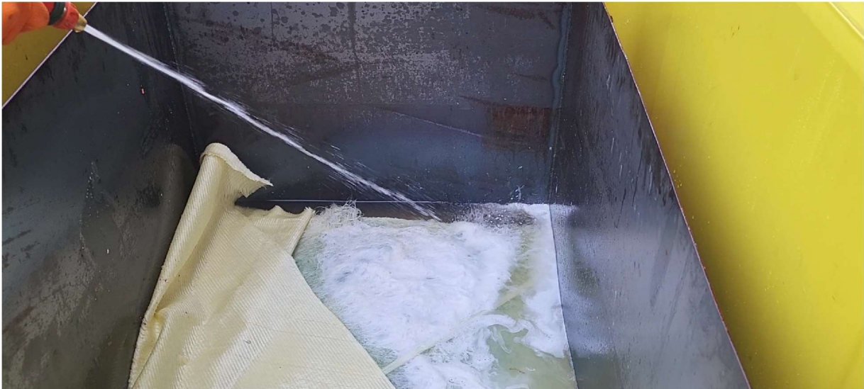
Figure 9: After PAA is pumped out, the water is added to the reactor to remove the residual acetic acid and hydrogen peroxide. The 2 nd layer of the fragment - glass fiber sheet – is visibly self-delaminated
