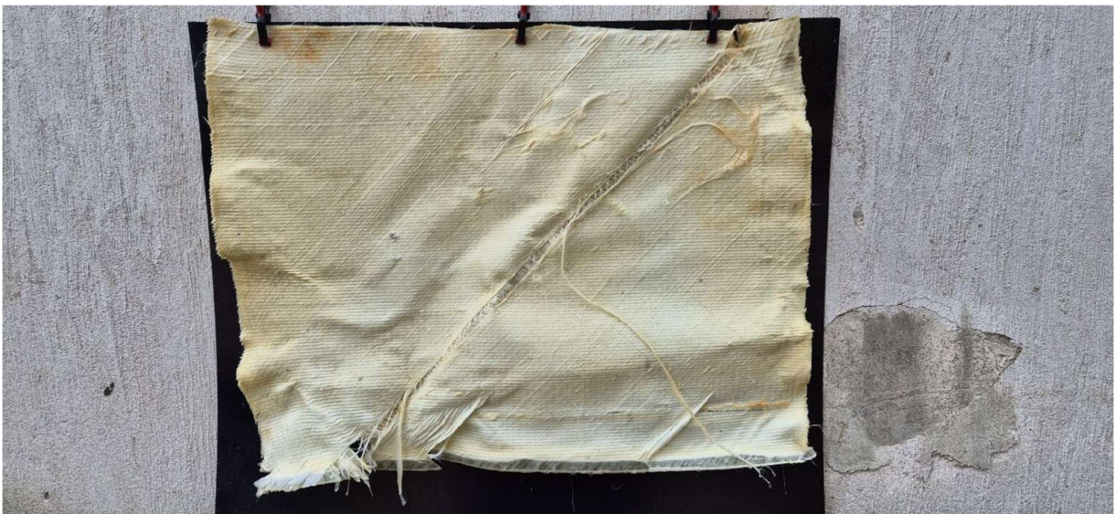
Figure 12: The 2 nd layer (glass fiber sheet) is removed from the reactor and dried
