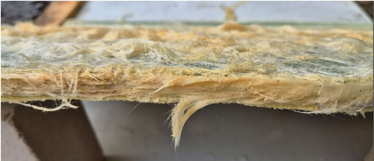
Figure 13: Intermedia layers, including the glass fiber wool, are being dried and visible
