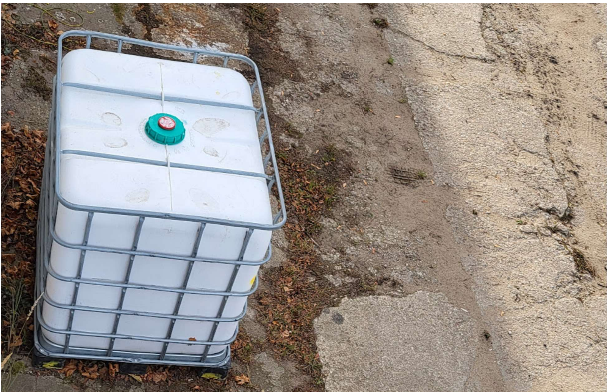
Figure 14: The contaminated PAA is stored in a vented HDPE container, dissolved with water 4:1. Over time, it decomposes into its constituent products—acetic acid, hydrogen peroxide, and oxygen
