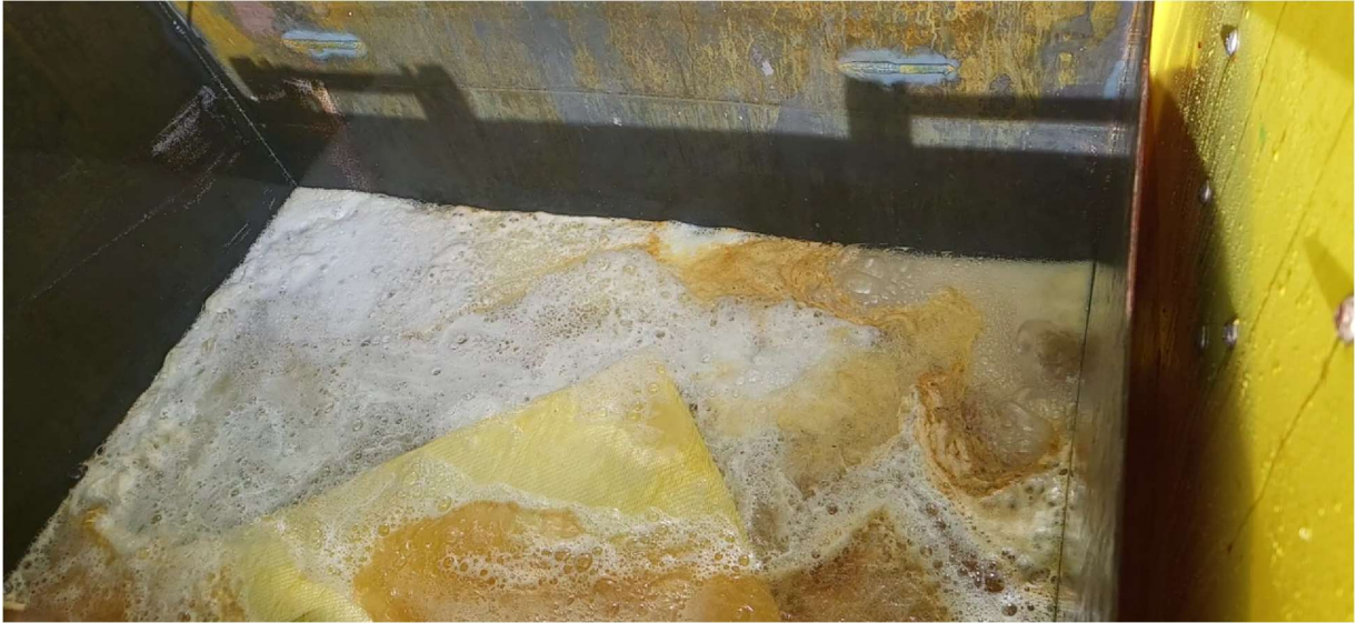
Figure 11: The exothermic reaction is causing a highly turbulent flow thus ensuring removal of residual epoxy compounds that might have remained on the glass fiber sheet
